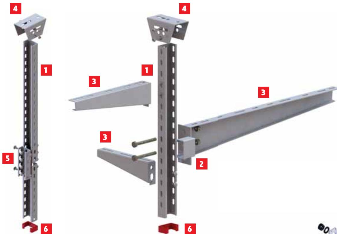
**PRINCIP MONTAŽE NA U PROFIL / THE PRINCIPLE OF THE MOUNTING CABLE TRAYS AGAINST THE U PROFILE**
